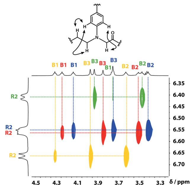
Fig. 3 Part of the  $^1\text{H}$ - $^1\text{H}$  NOESY (500 MHz,  $\text{CDCl}_3$ , 298 K, ca. 5 mM) spectrum of the ADAD 4-mer showing cross-peaks with the R2  $^1\text{H}$  signal. Signals due to different residues are distinguished by colour.
