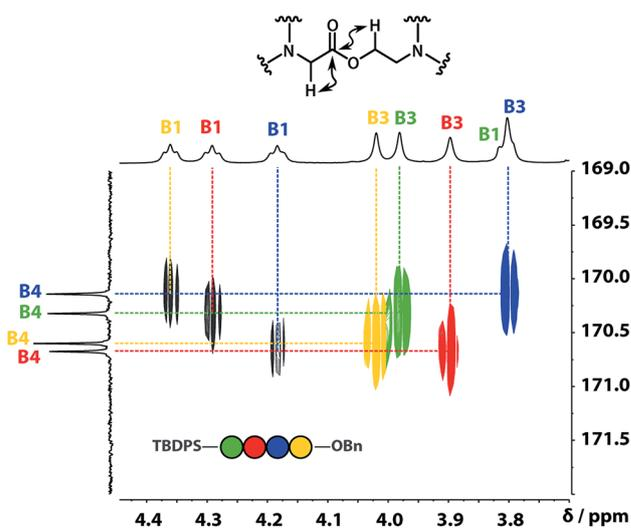
Fig. 4 Part of the  $^1\text{H}$ - $^{13}\text{C}$  HMBC (500 MHz,  $\text{CDCl}_3$ , 298 K, ca. 5 mM) spectrum of the ADAD 4-mer showing cross-peaks with the B4  $^{13}\text{C}$  signal. This spectrum established the connectivity of the residues illustrated.
