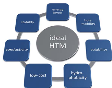
Fig. 2 Schematic representation of summarized HTM properties required for PSCs in an ideal case.
