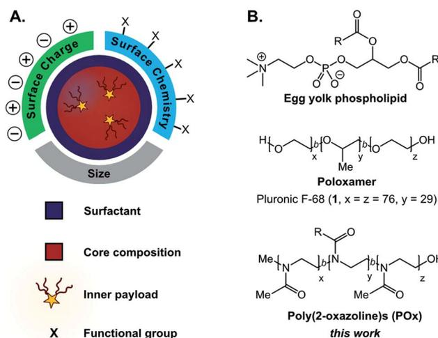
**Fig. 1** (A) Surfactants dictate the size, charge, and surface chemistry of emulsions. Emulsion cores can be composed of several liquid phases (e.g. oil, perfluorocarbon). Payloads can be solubilized in the emulsion core and functional groups can be appended on the surface. (B) Selected surfactants for emulsion formation, including poly(2-oxazoline) surfactants presented herein.
