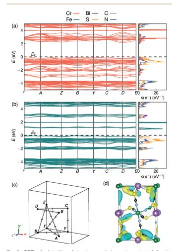
Fig. 6 DFT calculated band structure and element-projected density of states for (a) Cr[Bi(SCN)<sub>6</sub>] and (b) Fe[Bi(SCN)<sub>6</sub>]. Both spin channels have been plotted at once, as the differences between them are minor. (c) Reciprocal space path used for band structure calculations. (d) Kohn-Sham orbital for Cr[Bi(SCN)<sub>6</sub>] at the valence band maximum, showing the localised nature of the valence band states, viewed along the [100] direction. Atoms are coloured as in Fig. 3.
