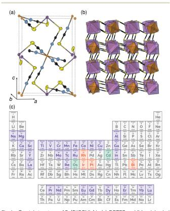
Fig. 1 Crystal structure of Fe[Bi(SCN)<sub>6</sub>] in (a) ORTEP and (b) polyhedral representations. Atoms are coloured as follows Bi, purple; Fe, brown; S, yellow; C, black and N, blue. (c) The periodic table coloured by whether the homoleptic metal hexathiocyanate anion is known. If  $[M(NCS)]^{n-}$  is known in the CSD or ICSD structural database, the element is coloured indigo, if  $[M(NCS)]^{n-}$  is known, it is coloured orange, if both are known, it is coloured green.
