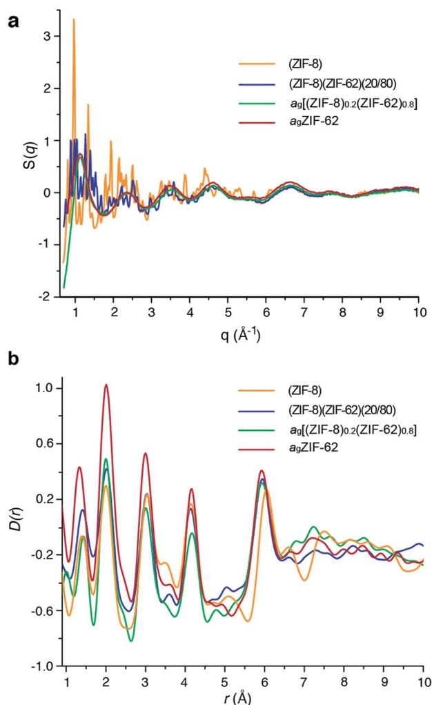
Fig. 4 (a) Structure factors  $S(q)$  of (ZIF-8)(ZIF-62)(20/80),  $a_g[(ZIF-8)_{0.2}(ZIF-62)_{0.8}]$  and ZIF-8, alongside that of  $a_g$ ZIF-62 from a previous publication.<sup>46</sup> (b) Corresponding X-ray pair distribution functions  $D(r)$ .
