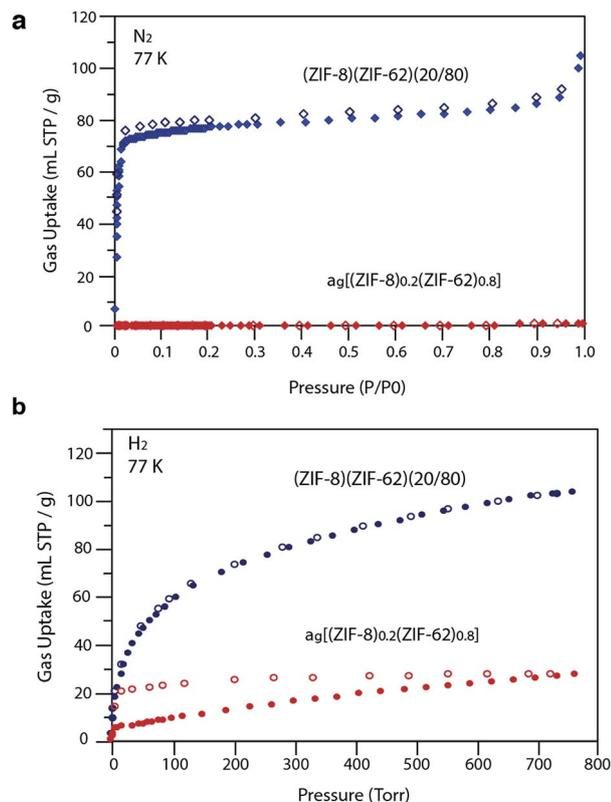
Fig. 6 (a) N<sub>2</sub> at 77 K and (b) H<sub>2</sub> at 77 K gas isotherms for the zinc-based crystalline mixtures and glasses. Closed symbols represent adsorption isotherms and open symbols represent desorption isotherms.
