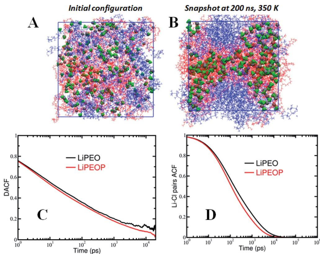
Fig. 4 (A) Initial configuration and (B) equilibrated snapshot at 200 ns of the PEO-PDMS-LiClO<sub>4</sub> electrolyte at 350 K. (C) Dihedral angle autocorrelation function (DACF) of the PEO polymer backbone to understand the effect of PDMS on polymer dynamics, and (D) Li-Cl ion pairs autocorrelation function (ACF).
