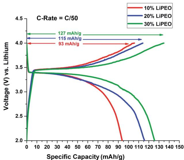
Fig. 3 Effect of salt concentration in PEO electrolyte on 2<sup>nd</sup> cycle of charge discharge of  $\text{LiFePO}_4$  half cells at 60 °C.
