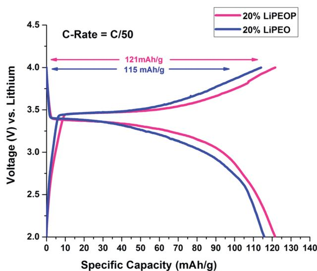
Fig. 6 Charge-discharge cycles showing the effect of addition of PDMS in 20% PEO electrolyte on the 2<sup>nd</sup> cycle of charge-discharge of LiFePO<sub>4</sub> half cells at  $60^\circ\text{C}$ .
