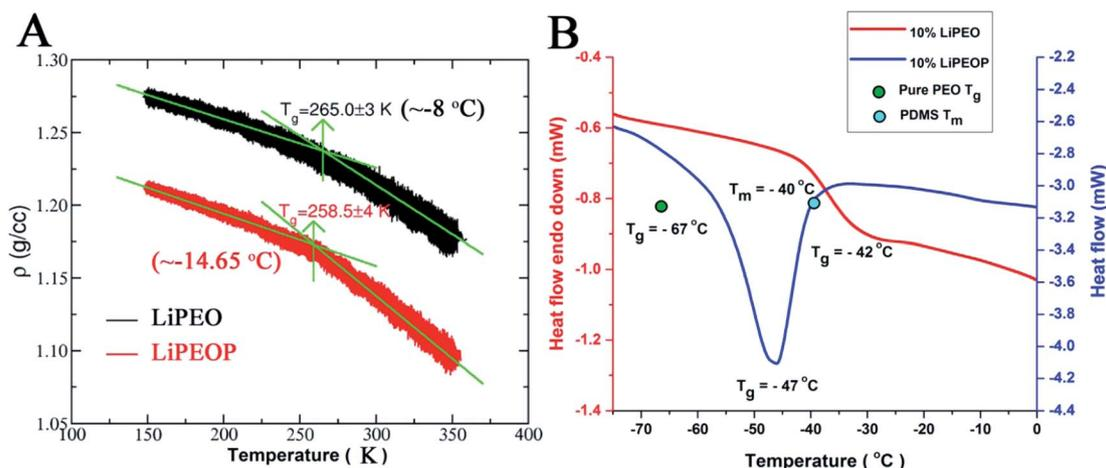
Fig. 5 The theoretical (A) and experimental (B) DSC curves of LiPEO and LiPEOP. The  $T_g$  of the pure PEO (the reported value) is denoted by the green dot in the (B). The sky blue dot in the figure is the  $T_m$  of the PDMS.
