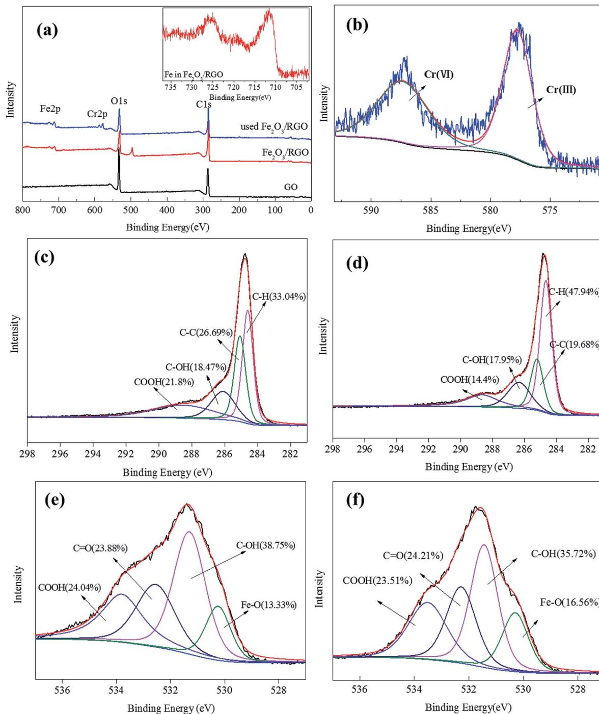
Fig. 6 The spectra survey scans of GO, Fe<sub>2</sub>O<sub>3</sub>/rGO and used Fe<sub>2</sub>O<sub>3</sub>/rGO (a); Cr 2p spectra of used Fe<sub>2</sub>O<sub>3</sub>/rGO (b); C 1s spectra of unused Fe<sub>2</sub>O<sub>3</sub>/rGO (c); C 1s spectra of used Fe<sub>2</sub>O<sub>3</sub>/rGO (d); O 1s spectra of unused Fe<sub>2</sub>O<sub>3</sub>/rGO (e); O 1s spectra of used Fe<sub>2</sub>O<sub>3</sub>/rGO (f).
