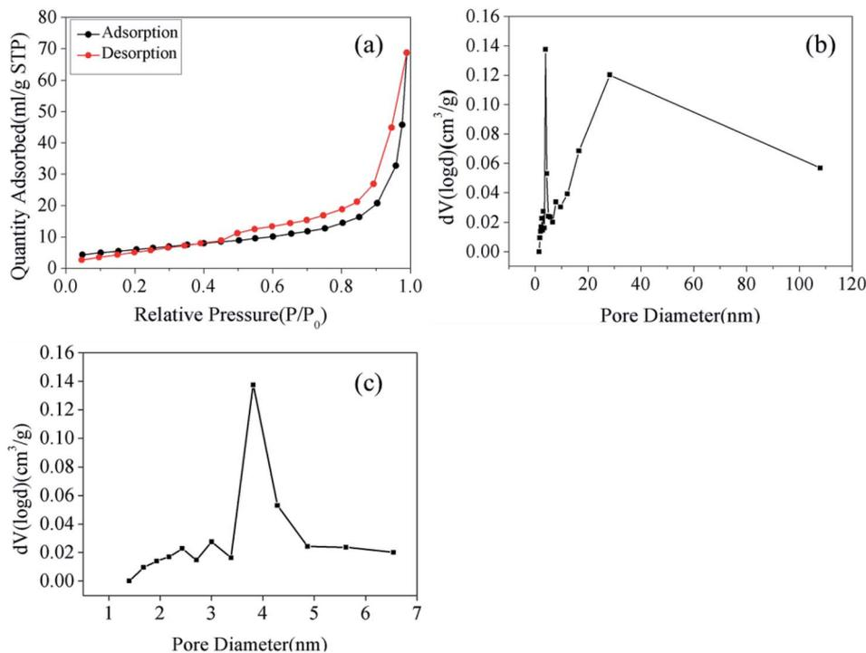
Fig. 3  $\text{N}_2$  adsorption/desorption isotherms (a); pore size distribution of  $\text{Fe}_2\text{O}_3/\text{rGO}$  (b); pore size distribution of  $\text{Fe}_2\text{O}_3/\text{rGO}$  ranging from 1 to 7 nm (c).
