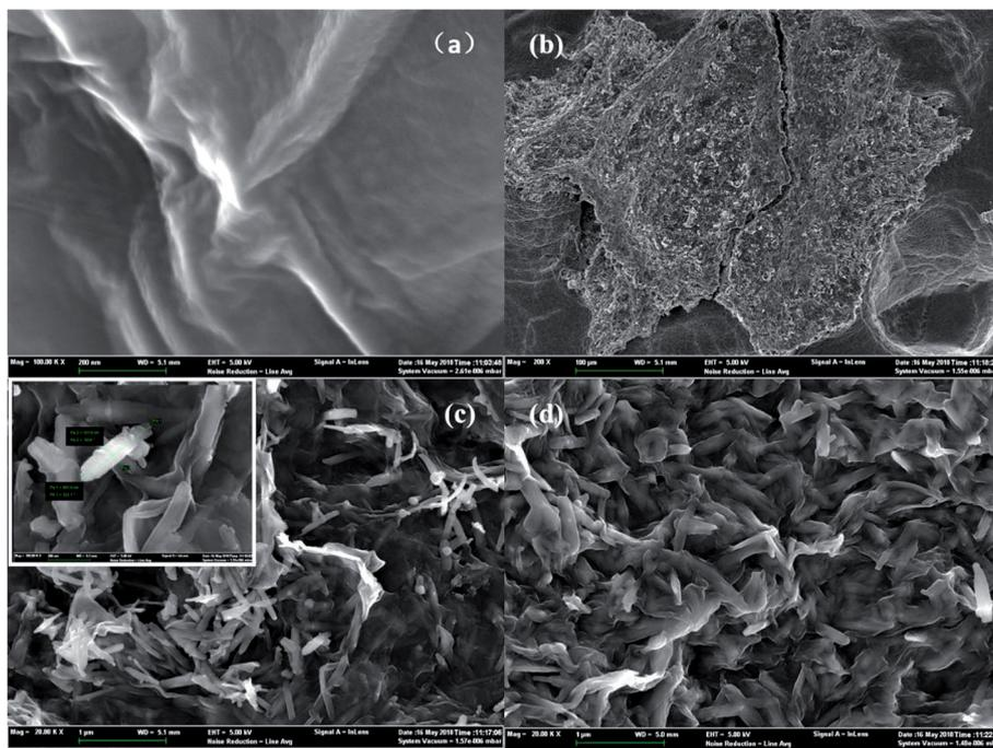
Fig. 2 SEM of GO (a); low-magnifications SEM images of unused  $\text{Fe}_2\text{O}_3/\text{rGO}$  (b); high-magnifications SEM images of unused  $\text{Fe}_2\text{O}_3/\text{rGO}$  (c); used  $\text{Fe}_2\text{O}_3/\text{rGO}$  (d).
