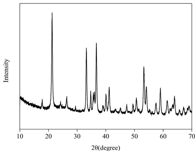
Fig. 4 The XRD pattern of  $\text{Fe}_2\text{O}_3/\text{rGO}$ .
