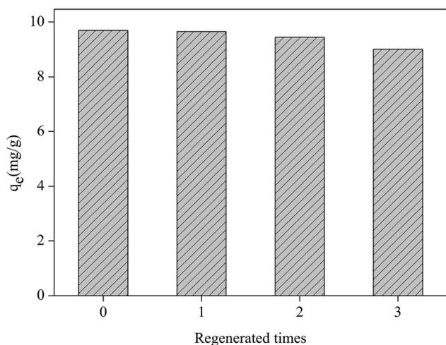
Fig. 10 Regeneration test of the  $\text{Fe}_2\text{O}_3/\text{rGO}$  (dosage =  $0.2 \text{ g L}^{-1}$ ;  $C_0 = 5.0 \text{ mg L}^{-1}$ ;  $V = 50 \text{ mL}$ ;  $t_{\text{removal}} = 3 \text{ h}$ ;  $0.1 \text{ mol L}^{-1}$  NaOH, desorption agent;  $t_{\text{desorption}} = 3 \text{ h}$ ).
