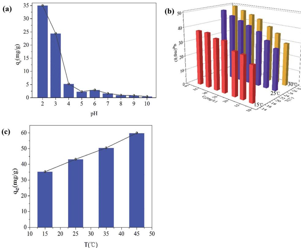
Fig. 9 Effect of pH on Cr(vi) removal ( $C_0 = 16.63 \text{ mg L}^{-1}$ ; dose of  $\text{Fe}_2\text{O}_3/\text{rGO} = 0.4 \text{ g L}^{-1}$ ;  $T = 25 \pm 1 \text{ }^\circ\text{C}$ ;  $t = 36 \text{ h}$ ; 140 rpm) (a); effect of the initial Cr(vi) concentration (b); effect of the temperatures (c) (dose of  $\text{Fe}_2\text{O}_3/\text{rGO} = 0.4 \text{ g L}^{-1}$ ; pH = 2.2;  $t = 36 \text{ h}$ ; 140 rpm).
