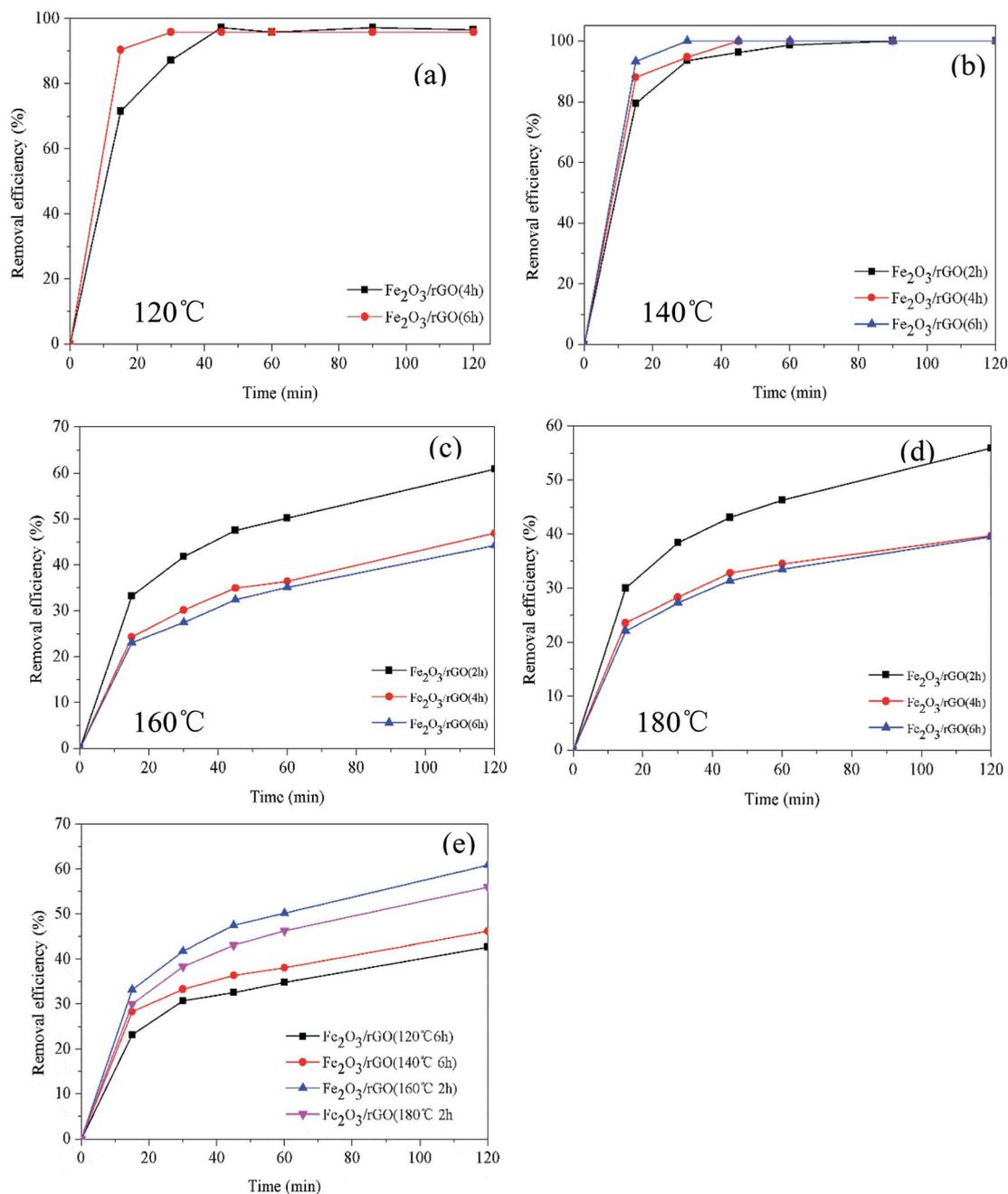
**Fig. 1** Effect of preparation time on Cr(vi) removal at different temperatures ( $C_0 = 2.0 \text{ mg L}^{-1}$ ; dosage =  $0.5 \text{ g L}^{-1}$ ;  $V = 100 \text{ mL}$ ;  $t = 2 \text{ h}$ ) (a) and (b); ( $C_0 = 5.0 \text{ mg L}^{-1}$ ; dosage =  $0.2 \text{ g L}^{-1}$ ;  $V = 100 \text{ mL}$ ;  $t = 2 \text{ h}$ ) (c) and (d); comparison of the best samples in each group (e) ( $C_0 = 5.0 \text{ mg L}^{-1}$ ; dosage =  $0.2 \text{ g L}^{-1}$ ;  $V = 100 \text{ mL}$ ;  $t = 2 \text{ h}$ ).
