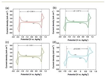
Fig. 1 CV curves of (a) 0.01 M BP/0.01 M DBB, (b) 0.01 M 44DMBP/ 0.01 M DBB, (c) 0.01 M 44DMOBP/0.01 M DBB, and (d) 0.01 M 4NBP/  $0.01 \,\mathrm{M}$  DBB in  $0.1 \,\mathrm{M}$  TEAPF<sub>6</sub>/MeCN at the scan rate of  $0.5 \,\mathrm{V} \,\mathrm{s}^{-1}$ . Arrows mark the scan directions.
