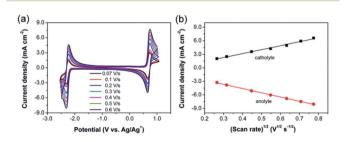
Fig. 3 (a) CV curves of 44DMBP/DBB in 0.1 M TEAPF<sub>6</sub>/MeCN at scan rates ranging from 0.07 to 0.6 V s<sup>-1</sup>. (b) Plot of peak current density as a function of (scan rate)<sup>1/2</sup> for the 44DMBP analyte and DBB catholyte
