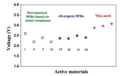
Fig. 2 Comparison of open-circuit voltage of cells in this work and that in literature. The numbers inset are the reference numbers.7-9,15-17,19,23
