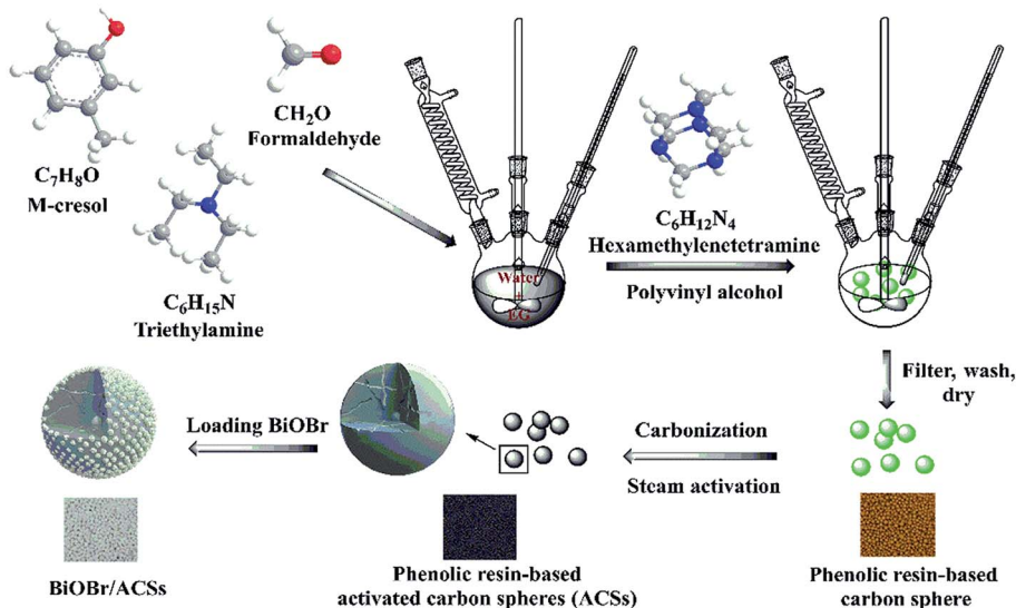
Scheme 1 Preparation process of BiOBr/ACSs.
