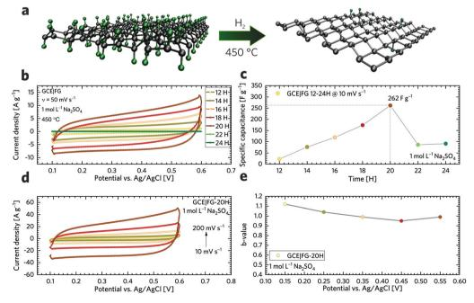
Fig. 4 (a) Scheme of fluorographene synthesis. (b) CVs of GCEs modified with fluorographene samples recorded at a constant scan rate of 50 mV s<sup>-1</sup>. (c) Change of specific capacitance of FG samples with increasing time of synthesis. (d) CVs for the GCE modified with GF-20 H at different potential scan rates ranging from 10 to 200 mV s<sup>-1</sup>. (e) Variation of the b-value with the potential for the FG-20H sample.
