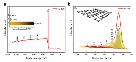
Fig. 3 (a) XPS survey and elemental analysis (inset) of the FG-20H sample. (b) HR-XPS spectra of C 1s from the FG-20H sample.
