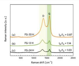
Fig. 2 Raman spectra of (a) FG-20H, (b) FG-12H, (c) and FG-24H samples and the corresponding intensity ratios  $I_{\rm D}/I_{\rm G}$ .
