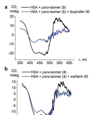
Fig. 7 Initial ICD spectra of the para-isomer 3-HSA assembly and those after addition of a 50-fold excess of albumin site-specific drugs ibuprofen (a) and warfarin (b)
