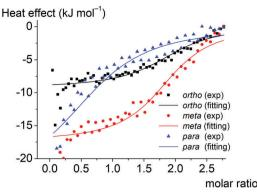
The experimental (depicted in the points) and fitted (depicted in the solid lines) plots of the binding heat effect versus the BSA-toclathrochelate molar ratio for the ortho-, meta- and para-substituted hexacarboxyphenyl-terminated iron(II) clathrochelates 1-3 as guests.
