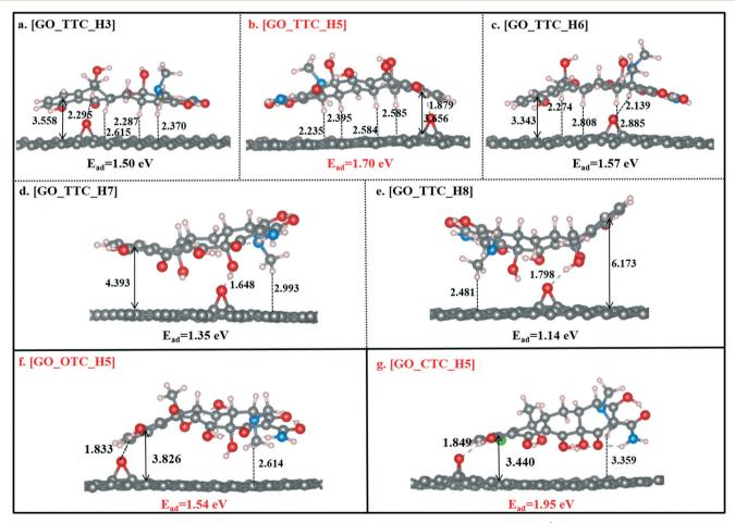
Fig. 3 The optimized geometries of GO\_TTC, GO\_OTC, and GO\_CTC complexes, bond lengths are in Å (the vertical distance refers to the distance between the centroid of benzene of TCs to the basal plane of GO).
