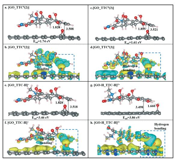
Fig. 7 The optimized geometries of [GO\_TTC<sup>0</sup>(2)] (a), [GO\_TTC<sup>0</sup>(3)] (c), [GO\_TTC-H]<sup>+</sup> (e), and [GO-H\_TTC-H]<sup>2+</sup> (g) systems and their charge density difference plots (b, d, f and h).
