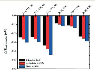
Fig. 8 The solution effect ( $\Delta E_{\text{solvation}}$ ) in different solvents for GO\_TC and RGO\_TC systems.
