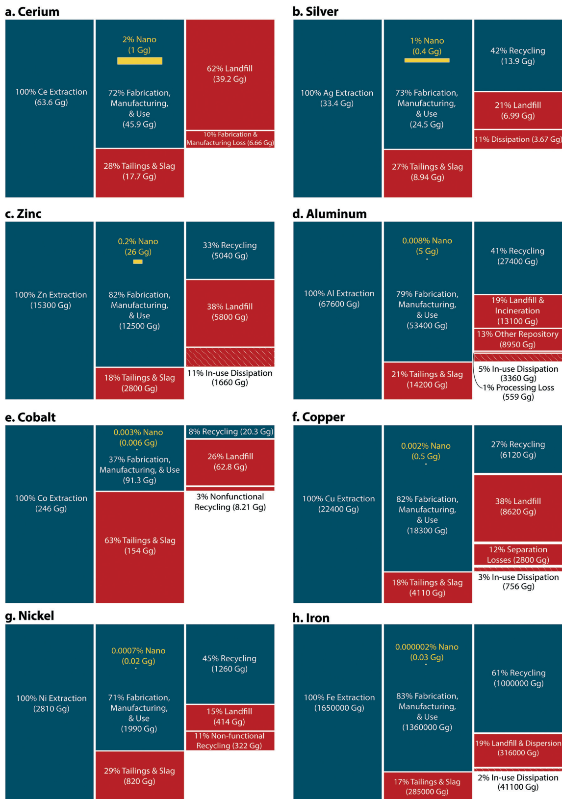
Fig. 4 Global material efficiencies across one life cycle of the particular element, from extraction of ore to end-of-life (left to right): production, fabrication, manufacturing, and use, and waste management/end-of-life. Red: losses from the anthropogenic cycle, where striped areas are losses during the use phase; blue: flows of metal to the anthropogenic cycle; yellow: engineered nanomaterial. Areas of rectangles reflect the magnitude of material flows as the percent of extracted ore in Gg of metal content, based on 2014 production volumes. Nanomaterial flows are based on high production volume estimates for 2014. All masses are in metal content of the particular element. All masses are rounded to 3 significant digits with the exception of nanomaterial flows. A glossary of terms is provided in the ESI† Table S1.
