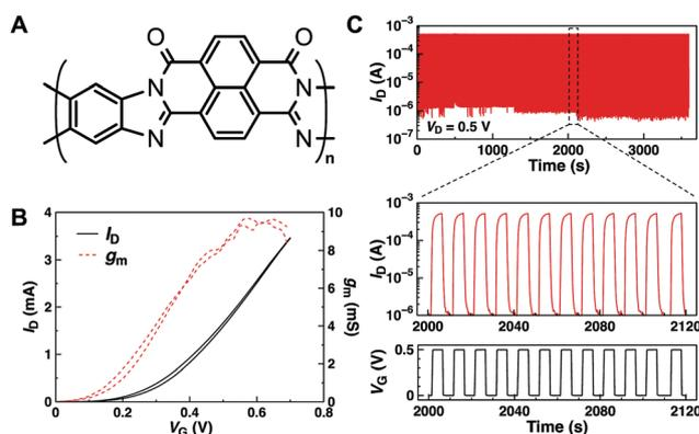
Fig. 4 (A) Chemical structure of BBL. (B) n-Type transfer curve (black) and transconductance (red dotted) of a 180 nm-thick BBL OECT measured at  $V_D = 0.6\text{ V}$  in 0.1 M NaCl. (C) Stability test of BBL OECT under sequential square wave gate voltage pulse for 1 h in water. Reprinted with permission from ref. 58 copyright The Authors.
