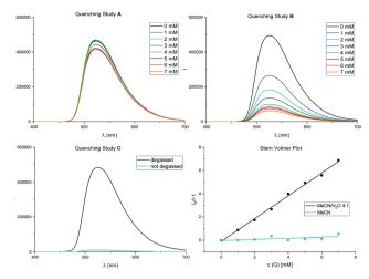
Fig. 2 Stern-Volmer guenching studies. Fluorescence spectra for fac-Ir(ppy)<sub>3</sub> (50  $\mu$ M) with increasing amounts of  $\alpha$ -acetoxy acetophenone 1 (0-7 mM) as quencher. Quenching study A: in MeCN; quenching study B: in MeCN/H2O 4:1; quenching study C: presence of oxygen. For further details, see ESI.†
