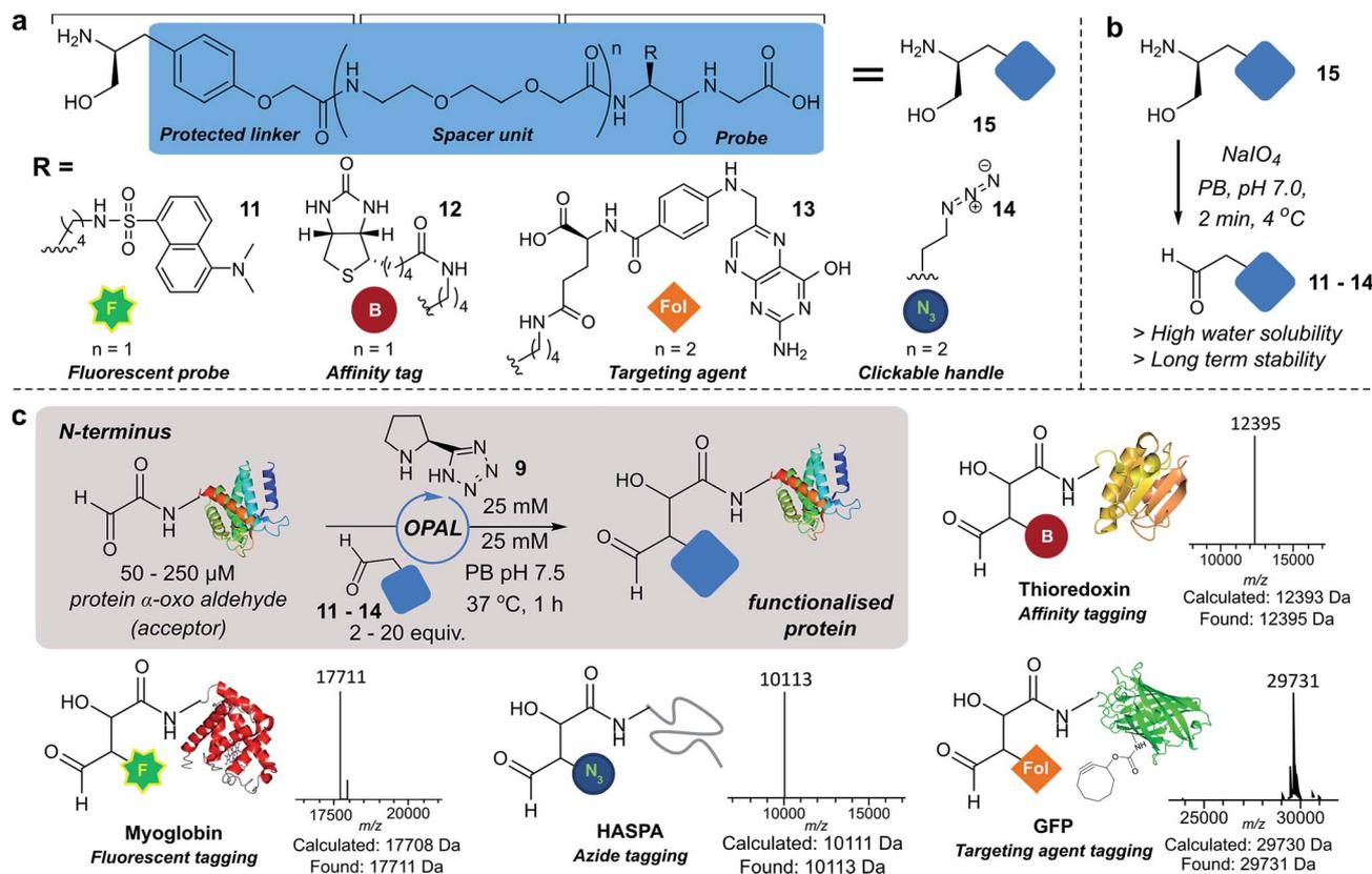
Fig. 3 (a) OPAL probe precursors bearing functional tags. (b) Mild  $\text{NaIO}_4$  unmasking of  $\alpha$ -aryl aldehyde probes. (c) OPAL functionalization of N-terminal  $\alpha$ -oxo aldehyde containing proteins (50–250  $\mu\text{M}$ ), using probes 11–14 (0.5–1.5 mM).
