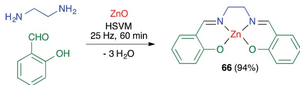
Scheme 46 Mechanochemical synthesis of a zinc-salen complex.
