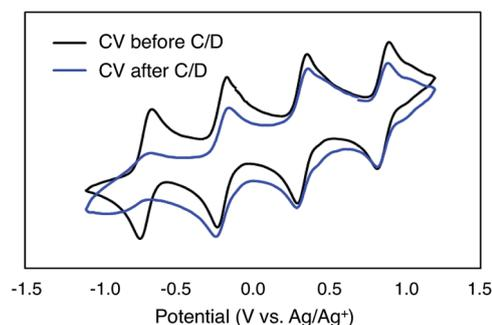
Fig. 4 CV of complex **1-V<sub>6</sub>O<sub>7</sub>(OMe)<sub>12</sub>** before and after cycling.
