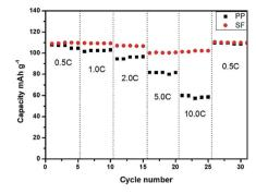
Fig. 10 The rate performance of the batteries with PP separator and SF separator.
