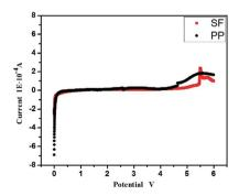
Fig. 7 The linear sweep voltammograms of PP and SF with Li and stainless steel electrode from 0 V to 6 V.
