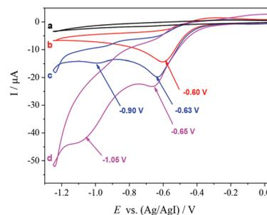
Fig. 1 Cyclic voltammograms recorded on a Pt electrode at 100 mV s<sup>-1</sup> in: (a) DMF containing 0.07 M Bu<sub>4</sub>NPF<sub>6</sub>; (b) solution (a) after addition of 2 mM [(R)-BINAP]Pd(OAc)<sub>2</sub>; (c) solution (b) after addition of 20 mM **1b**; (d) solution (c) saturated with CO<sub>2</sub>.
