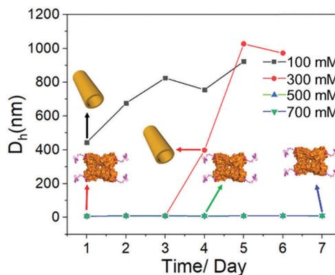
**Fig. 5** Time-dependent DLS results of SBA/R3GN with different concentrations (100 mM, 300 mM, 500 mM and 700 mM) of  $\text{Ca}(\text{NO}_3)_2$  at 4 °C (pH = 6.0, [SBA]: 0.1 mM and [R3GN]: 0.2 mM). The inset cartons correspond to the mixture state of SBA/R3GN at different incubation times and concentrations of  $\text{Ca}(\text{NO}_3)_2$  at 4 °C.
