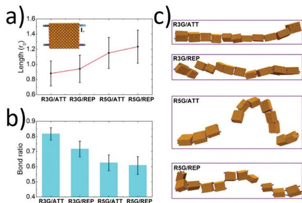
**Fig. 4** Simulation results of comparison of the stability of the protein chains in different cases. (a) The effective length (defined as the distance between the coating site and the terminal of ligands, see the inset) of the ligand in different cases. (b) The bond ratio (defined as the equilibrium bond number/the maximum bond number) in different cases. (c) Typical equilibrium snapshots of the protein chains in different cases in the simulations.
