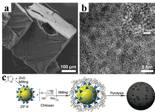
Fig. 7 (a) SEM image and (b) TEM image of ZnO QDs@porous carbon. Reproduced with permission.<sup>93</sup> Copyright 2013, American Chemical Society. (c) Synthetic route of ZIF-8@chitosan-800N. Reproduced with permission.<sup>94</sup> Copyright 2014, Royal Society of Chemistry.
