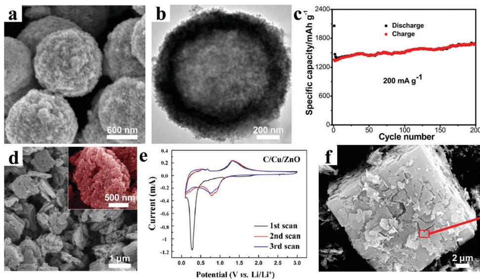
**Fig. 10** (a) SEM and (b) TEM images of sandwich-like Ag-C@ZnO-C@Ag-C hybrid hollow microspheres; (c) cycling performances at  $0.2 \text{ A g}^{-1}$ . Reproduced with permission.<sup>129</sup> Copyright 2015, American Chemical Society. (d) SEM image and (e) CV curves of the C/Cu/ZnO hybrids. Reproduced with permission.<sup>130</sup> Copyright 2014, American Chemical Society. (f) SEM image of the CZO@C. Reproduced with permission.<sup>131</sup> Copyright 2014, American Chemical Society.
