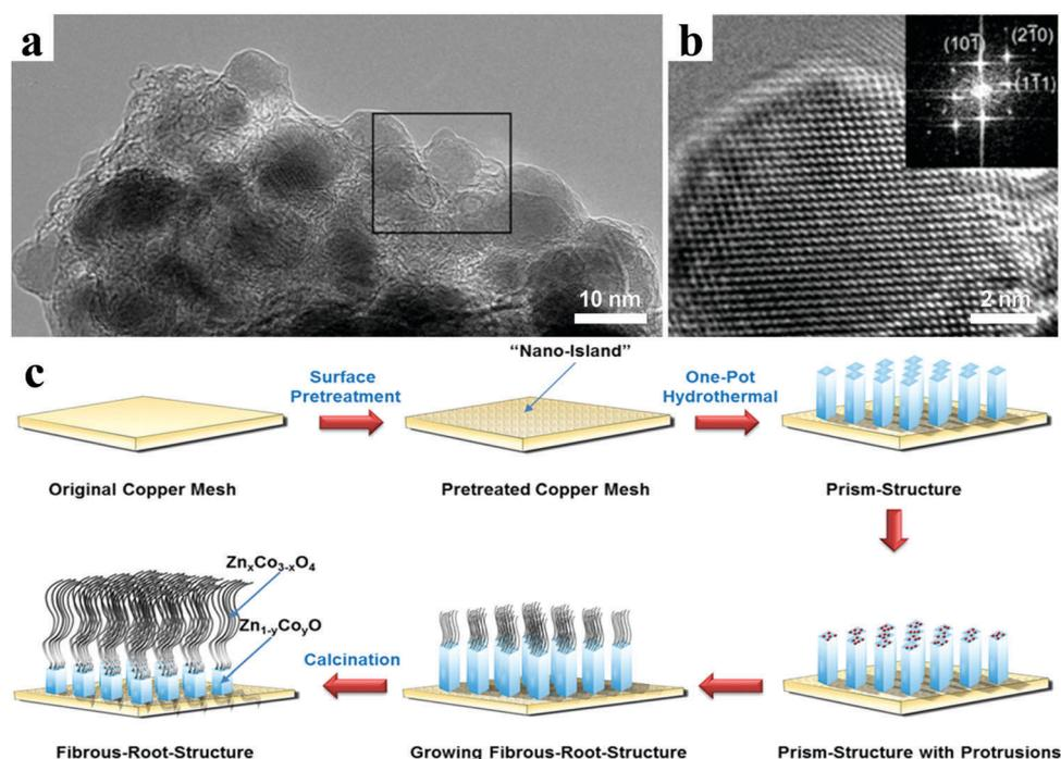
Fig. 11 (a) TEM and (b) HRTEM images of Fe-doped ZnO nanoparticles, inset in panel (b) showing the corresponding FT. Reproduced with permission.<sup>132</sup> Copyright 2013, American Chemical Society. (c) Preparation procedure of Zn<sub>x</sub>Co<sub>3-x</sub>O<sub>4</sub>@Zn<sub>1-y</sub>Co<sub>y</sub>O binary nanoarrays. Reproduced with permission.<sup>133</sup> Copyright 2016, American Chemical Society.
