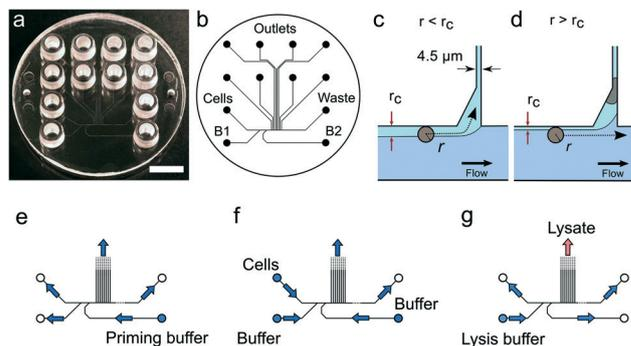
**Fig. 1** Device design and operation. (a) Image of the single use polymer device. Scale bar is 1 cm. (b) Microfluidics layout. (c) Conditions for cell trapping an unoccupied trap  $r < r_c$ . (d) The trapped cell reduces the flow through the trap such that for the next incoming cell,  $r > r_c$ . (e–g) Flow directions in the device under priming, cell capture and lysis.
