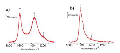
Fig. 4 Raman spectra of the carbon support, collected with the laser line at 514 nm (part a) and at 244 nm (part b) as exciting sources. Previously unpublished figure, reporting data published in ref. 1.
