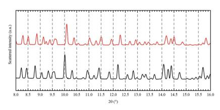
Fig. 10 X-ray diffraction patterns of the UiO-67-Pd sample taken during reduction in hydrogen at 33  $^{\circ}$ C (black) and 300  $^{\circ}$ C (red).
