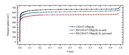
Fig. 11  $N_2$  adsorption isotherms of UiO-67 with 10% of modified ligands non-functionalized (black squares) and functionalized by Pd before (blue triangles) and after (red circles) activation in  $H_2$  at 300 °C.
