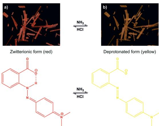
**Fig. 5** Colorimetric response the MR-rich solid **2** during the acid/base sensing process. a) Red-coloured zwitterionic MR-rich crystals of **2** changed into yellow-coloured anionic MR-rich solid when exposed to  $\text{NH}_3$  vapours and b) back from yellow to red when exposed to HCl vapours.
