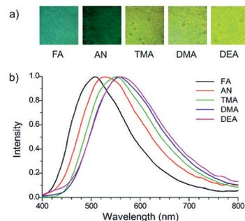
**Fig. 6** Luminescence turn on response of crystalline **2** to aniline derivatives: a) optical microscope images of **2** upon exposure to various aniline vapours under 365 nm UV lamp illumination and b) their normalized solid-state emission spectra ( $\lambda_{\text{exc}} = 365 \text{ nm}$ ).
