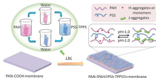
Scheme 1 Schematic model of LbL assembly membrane fabrication and pH-responsive structure of the TPPS assembly.
