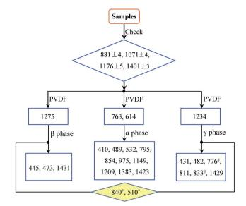
Fig. 1 Flow diagram for the identification of  $\alpha$ ,  $\beta$  and  $\gamma$  phases; 840\* and 510\* represents bands in the range of 837–841 and 508–512 cm<sup>-1</sup>, respectively; 776<sup>#</sup> and 833<sup>#</sup> reflects possible variations based on specific processes.
