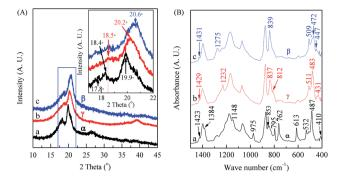
Fig. 4 XRD patterns (A) and FTIR spectra (B) of membranes cast from 8 wt% PVDF solution with  $V_{\rm NMP}/V_{\rm acetone}$  at 9/1: curve 'a' (black) for the sample dried at 150 °C; curve 'b' (red) for the sample dried at 40 °C; curve 'c' (blue) for the sample dried at 40 °C and drawn at 80 °C with a draw ratio of ca. 4.
