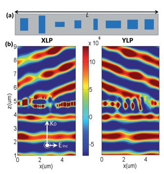
Fig. 2 (a) Schematic of eight resonators that provide a phase shift from 0 to  $2\pi$  for XLP incidence while conversely changing from  $2\pi$  to 0 for YLP incidence. (b) The extracted transmitted XLP (left) and YLP (right) electric field distributions of the designed metasurfaces under the normal incidence of  $45^\circ$  LP light at a wavelength of 1500 nm, respectively.
