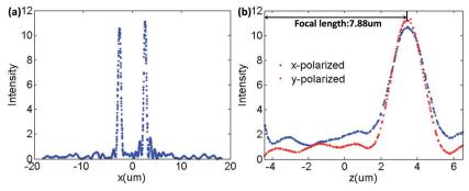
(a) The electric field intensity along the x-axis and (b) the z-axis at the focal plane.
