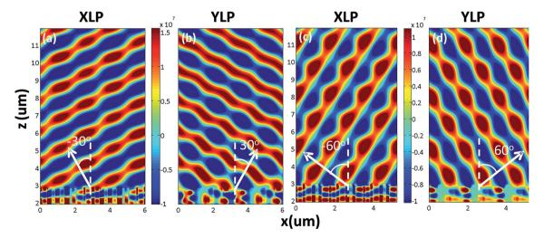
Fig. 3 Transmitted XLP (a and c) and YLP (b and d) electric field distributions of the metasurface illuminated with a normal incidences of 45° LP lights with the refractive angles of 30° (a and b) and 60° (c and d).
