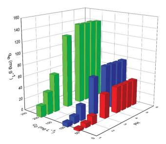
Fig. 5 The effect of initial solution pH on U(v1) removal by PAA hydrogels at various initial concentrations (60, 100 and 200 mg  $L^{-1}$ ). (Volume, 10 mL; adsorbent dose, 0.01 g; pH value, 1, 1.5, 2, 3, 4, 4.5, 5, 5.5; contact time, 180 min; temperature, 25 °C; rotating speed, 150 rpm). Note: data are presented as the mean  $\pm$  standard deviation of triplicate experiments.
