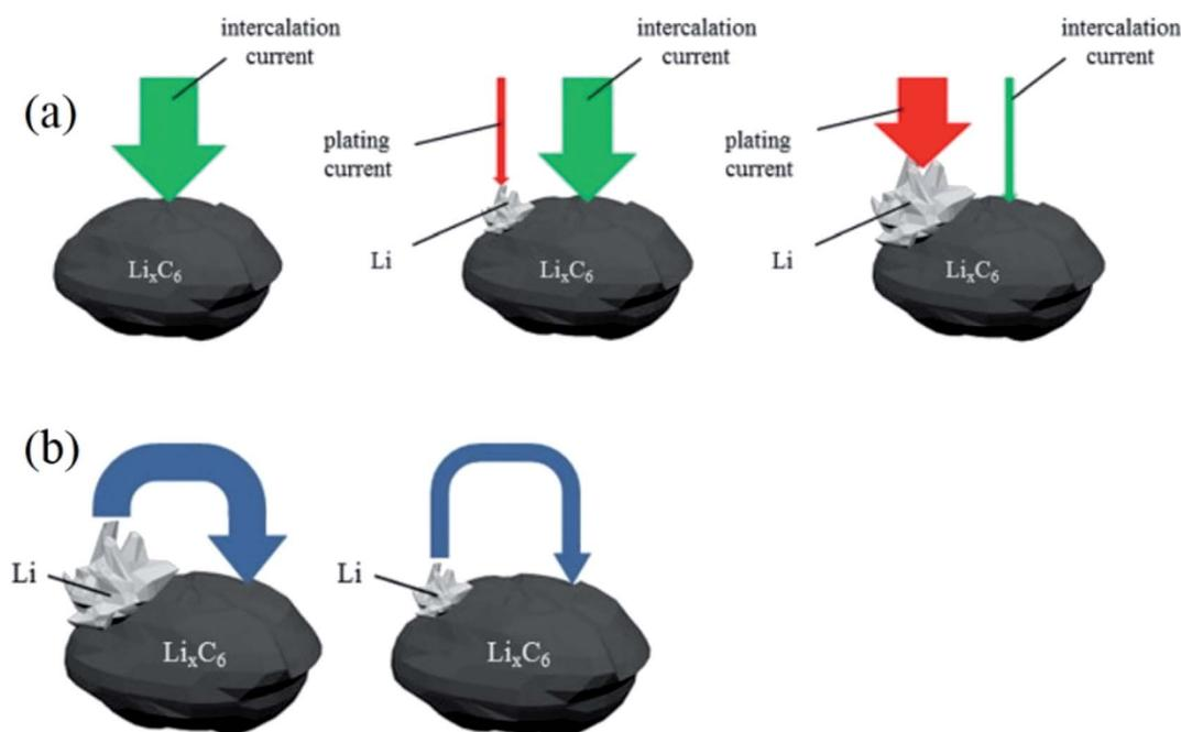
Fig. 1 Schematic of (a) the intercalation and plating currents during charging to higher states of charge, and (b) the re-intercalation of deposited lithium during rest (adapted from ref. 23).
