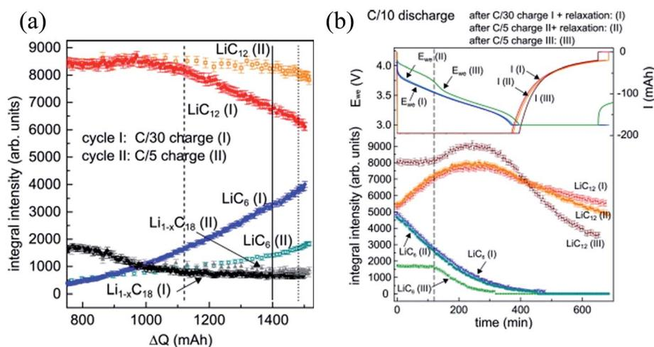
Fig. 5 (a) Integral reflection intensities of  $\text{LiC}_6$ ,  $\text{LiC}_{12}$ , and  $\text{Li}_{1-x}\text{C}_{18}$  during C/30 (I) and C/5 (II) charging; (b) integral reflection intensity of  $\text{LiC}_6$ ,  $\text{LiC}_{12}$ , and  $\text{Li}_{1-x}\text{C}_{18}$  during C/10 discharging after C/30 charging + 20 h rest (I), C/5 charging + 20 h rest (II) and C/5 charging + no rest (III) (adapted from ref. 95).
