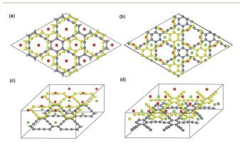
Fig. 3 Top view and 3D view of 2  $\times$  2 optimized Na-intercalated double-layer GY and GDY compound NaC<sub>4</sub> (a and c) and NaC<sub>6</sub> (b and d), respectively.
