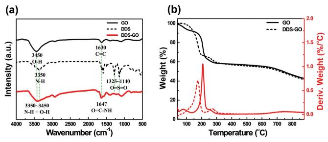
Fig. 2 (a) FT-IR spectra of GO, DDS, and DDS-GO. (b) TG-DTA curves of GO and DDS-GO during heating up to 900 °C under a N₂ atmosphere.
