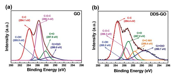
Fig. 3 XPS C 1s spectra of (a) GO and (b) DDS-GO. Deconvoluted curves represent the theoretical XPS spectra for different chemical bonds.
