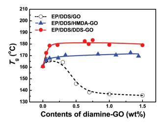
Fig. 6 Glass transition temperatures (Tq) of EP/DDS/diamine-GO nanocomposites.  $T_{\rm q}$  was estimated from the second heating DSC results of the EP/DDS/diamine-GO mixture.
