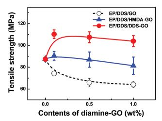
**Fig. 8** Tensile strengths of EP/DDS/diamine-GO nanocomposites. It was estimated by using a universal testing machine. Samples for measurements were prepared with 1.5 mm  $\times$  50 mm  $\times$  250 mm size, and tests were performed with a testing speed of 5 mm min<sup>-1</sup>.
