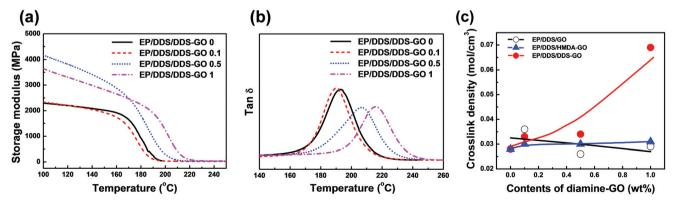
Fig. 7 DMA results of EP/DDS/diamine-GO nanocomposites. (a) Storage modulus, (b)  $\tan \delta$ , and (c) crosslink density of the EP/DDS/diamine-GO nanocomposites. Samples were tested in the temperature range of 30 to 260 °C at a scanning rate of 3 °C min<sup>-1</sup>. The crosslink density was calculated using storage modulus and tan  $\delta$  in the rubbery region of EP/DDS/diamine-GO nanocomposites.
