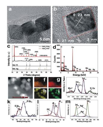
Fig. 2 Representative TEM image (a), HRTEM image (b), XRD pattern (c), EDX spectrum (d), high-angle annular dark-field scanning transmission electron microscope (HAADF-STEM) image (e), elemental maps for Mo (f), S (g), Pt (h) and Ag (i), peak-fitting XPS spectra of Mo 3d (j), S 2p (k), Pt 4f (l) and Ag 3d (m) regions of as-prepared MoS<sub>2</sub>-PtAg hybrid nanomaterials. The Cu, C, O in TEM-based EDX pattern (d) originated from carbon film supported by copper grids.
