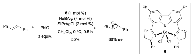
Scheme 5 Asymmetric epoxidation of an alkene with a Fe III carbazole-bis(oxazoline) complex.
