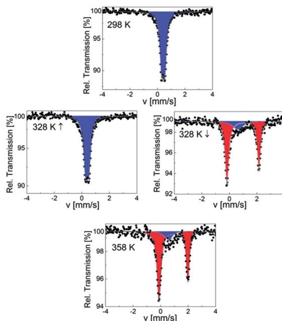
Fig. 7 Selected <sup>57</sup>Fe Mössbauer spectra of SCO-1@MCM; blue and red colors correspond to LS and HS doublets, respectively.
