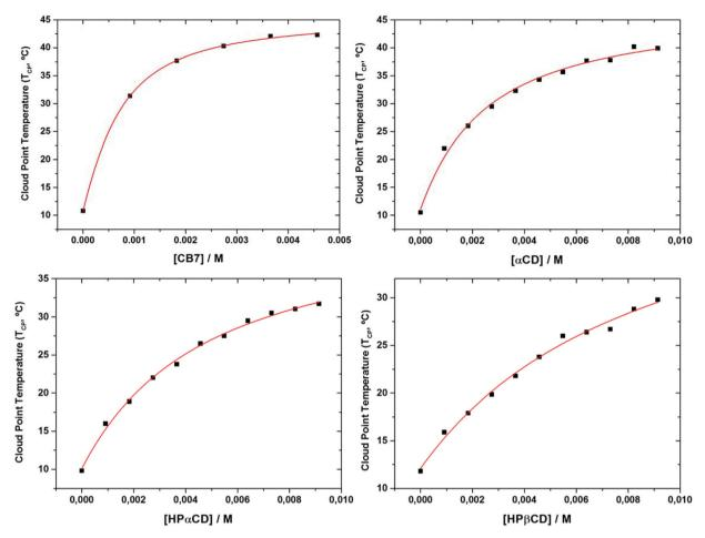
Fig. 7 Turbidimetry titration curves corresponding to 5 mg mL<sup>-1</sup> solutions of PEtOx<sub>90</sub>-ran-PNonOx<sub>12</sub>, and non-linear curve fitting based on egn (6). The average stability constants between the copolymer nonyl chains and cavitands follow the order: CB7  $\gg \alpha$ CD > HP $\alpha$ CD > HP $\beta$ CD.
