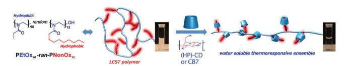
Fig. 1 An amphiphilic PEtOx<sub>90</sub>-ran-PNonOx<sub>12</sub> random copolymer was synthesized and its solubility properties studied in the presence of a range of different supramolecular host molecules. The picture describes the supramolecular complexation of the PEtOx<sub>90</sub>-ran-PNonOx<sub>12</sub> copolymer with cavitands resulting in the formation of thermoresponsive supramolecular complexes.
