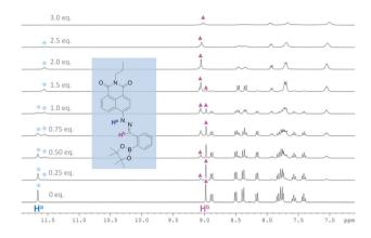
Fig. 8  $^{1}$ H NMR titration of probe 1 with TBAF in DMSO- $d_{6}$ . [1] = 20 mM.
