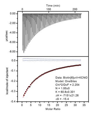
Fig. 3 ITC of Biotin[6]uril with KCNO in 100 mM phosphate buffer at pH 7.5 at 30 °C. Black: observed data, Red: fitted data, Blue: dilution contribution. K (M<sup>-1</sup>),  $\Delta H$  (cal mol<sup>-1</sup>) or  $\Delta S$  (cal mol<sup>-1</sup> deg<sup>-1</sup>).
