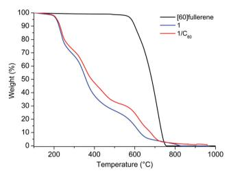
Fig. 3 TGA analysis (under a nitrogen atmosphere) of [60]fullerene, 1 and the 1/C<sub>60</sub> solution obtained by HSVM.
