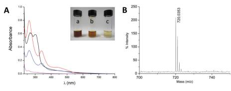
Fig. 2 (a) UV-Vis spectra of aqueous solutions of 1 (black) and 1/C<sub>60</sub> nanocomposites obtained by HSVM (red), manual grinding (blue) and sonication (pink). Inset: picture of the solutions obtained by HSVM (a), manual grinding (b) and sonication (c). (b) MALDI-TOF mass spectrum of the solution obtained by HSVM.
