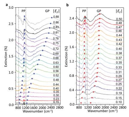
Fig. 2 (a) Extinction spectra ( $T = 1 - T(E_F)/T(CNP)$ ) of the graphene nanoribbon array at various values of  $E_F$  controlled by the ion-gel top gate. (b) Extinction spectra of the same device at various  $E_F$  values controlled by the back gate. These spectra were characterized before the ion-gel film was coated on the device. The absorption peaks of  $CO_2$  (ranging from 2244 to 2395 cm<sup>-1</sup>) in ambient air were replaced by straight lines.
