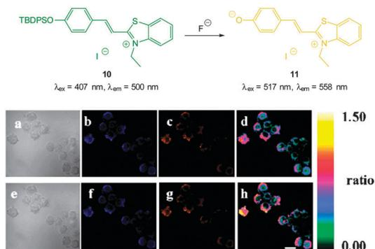
the amount of fluoride present in solution due to the linear relationship between the increase at 596 nm and the decrease at 438 nm. Imaging was performed in live HeLa cells and  $10 \mu\text{M}$  NaF was readily visualised using fluorescence microscopy.
