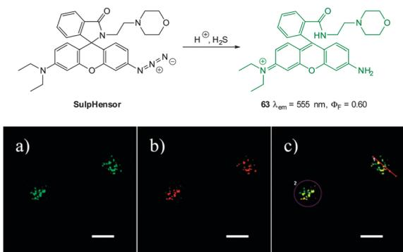
Fig. 61 Top: structure and reaction of **SulpHensor**. Bottom: HeLa cells stained with (a) LysoTracker Green (Ch1, green) and (b) **SulpHensor** (Ch2, red) with NaSH solution (c) overlay of (a) and (b). Scale = 10  $\mu\text{m}$ . Image reproduced with permission.<sup>233</sup>
