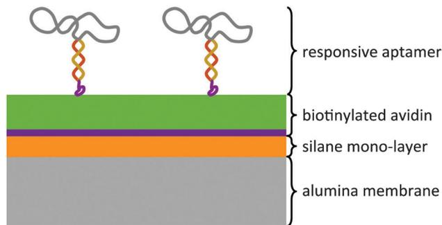
**Fig. 1** Modular architecture of the small-molecule stimuli-responsive membrane. The thickness of the support structure comprising the silane and avidin layers may be adapted depending on the size of the responsive receptor molecule (aptamer) and the pore size of the base material (AAO membrane).
