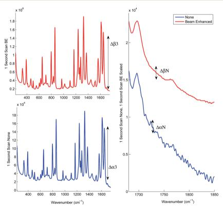
Fig. 3 1s scan time. The beam enhanced spectra have been reduced and scaled to the same relative intensity as the 'None'. Signal-to-noise analysis of the TRS spectra with and without the photon diode was performed to illustrate the improvement of SNR accompanying the boost of the signal intensity with photon diode.
