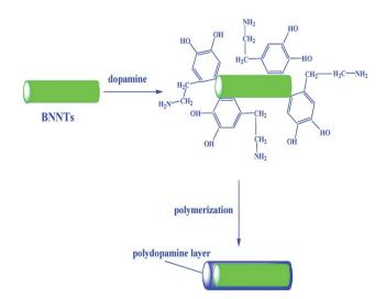
**Scheme 1** Schematic illustration of dopamine functionalization of BNNTs.
