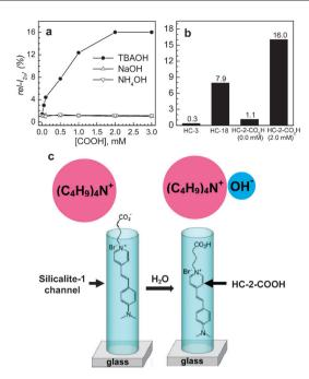
Fig. 9 Plots of  $I_{2\omega}$  versus [TBAOH], [NaOH], and [NH<sub>4</sub>OH], as indicated (a). Comparison of  $I_{2\omega}$  values of the primarily grown silicalite-1 films incorporating HC-3, HC-18, HC-2-COOH at [TBAOH] of 0.0 and 2.0 mM, respectively (b). A schematic illustration of orientation-controlled insertion of HC-2-COOH into the silicalite-1 channels with the tail first induced by the carboxylate-tetrabutylammonium ion pairing. (Adopted from ref. 49.)
