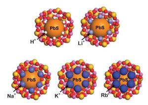
**Fig. 16** Schematic illustration of PbS-QD containing zeolite Y supercages with different counter cations: H<sup>+</sup>, Li<sup>+</sup>, Na<sup>+</sup>, K<sup>+</sup>, and Rb<sup>+</sup>, respectively.
