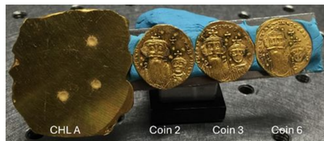
Figure 1. CHLA, and struck obverses of three gold solidi minted in Constantinople by the emperors Constans II and Constantine IV analysed with HERFD-XRF imaging and HERFD-XANES. Each coin is \sim 2 cm dia.
