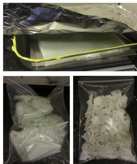
Fig. 10 Demonstration of fiber (bottom left) and polymer (bottom right) recovery by dissolution from a glass-fiber-reinforced composite (top) using Elium as the resin. Reproduced from ref. 102 with permission from Elsevier, J. Cleaner Prod. , 2019, 209 , 1252–1263, copyright 2019.
