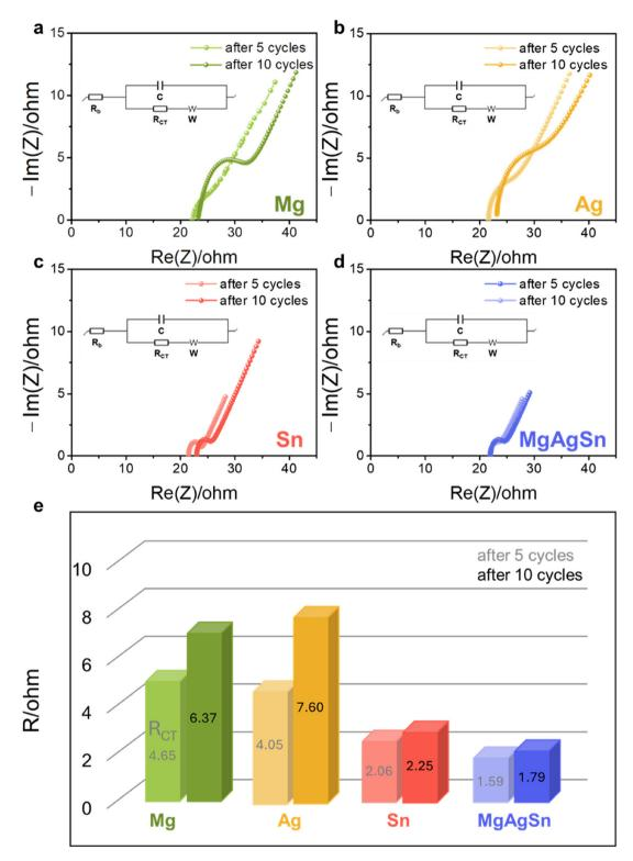
Fig. 3 Half-cell EIS analysis after Li plating-stripping. Nyquist plots and the corresponding equivalent circuits of the (a) Mg, (b) Ag, (c) Sn, and (d) MgAgSn half-cells after 5 and 10 cycles of Li plating-stripping. (e) Charge transfer resistance ( $R_{CT}$ ) values extracted from the EIS data.
