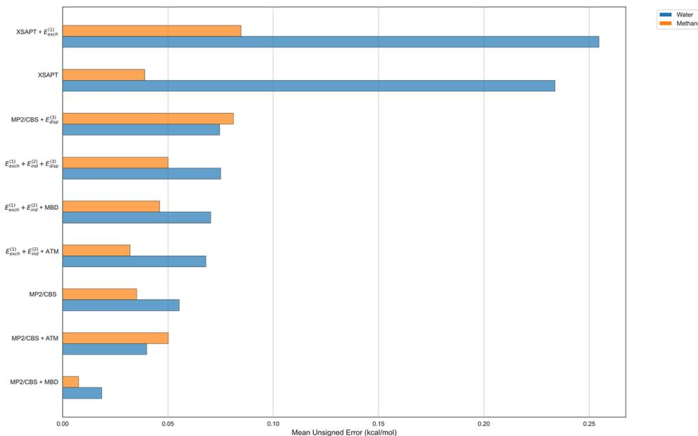
**Fig. 8** Mean unsigned errors (MUE, kcal mol<sup>-1</sup>) of various nonadditive three-body interaction energy estimates relative to the benchmark CCSD(T)-level  $E_{\text{int}}^3$  values. The corrections  $E_{\text{exch}}^{(1)}$ ,  $E_{\text{ind}}^{(2)}$ , and  $E_{\text{disp}}^{(3)}$  are taken from three-body SAPT(DFT), and their sum  $E_{\text{exch}}^{(1)} + E_{\text{ind}}^{(2)} + E_{\text{disp}}^{(3)}$  is by definition the SAPT(DFT) three-body interaction energy.
