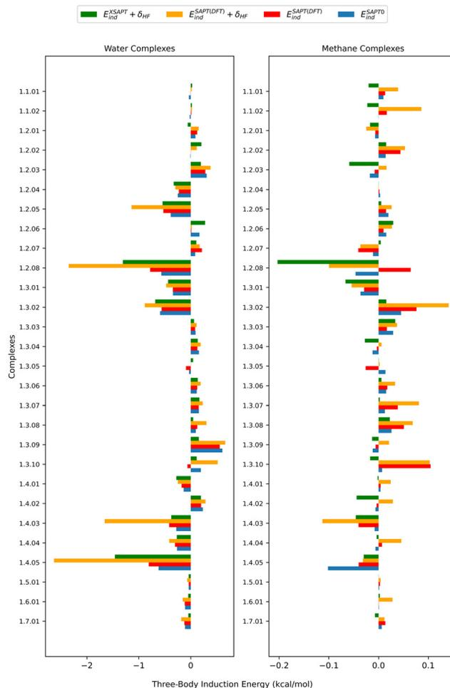
Fig. 5 Comparison of the nonadditive three-body induction energies for the systems with chlorine as the XB donor, predicted by SAPT0, XSAPT, and SAPT(DFT). The system labels are defined in the SI; the first '1.' part denotes chlorine. Note the different horizontal scale in the left and right panels.
