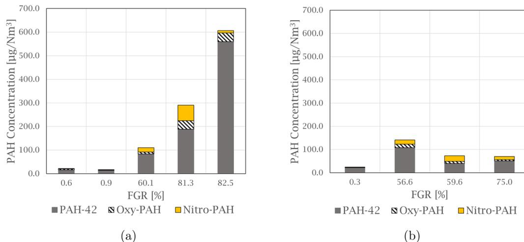
Fig. 1 Graphs showing the total PAH-42, oxy- and nitro-PAH concentrations in the off-gas at varying FGR levels for experiments at (a) 1000 Nm<sup>3</sup> h<sup>-1</sup> and (b) 500 Nm<sup>3</sup> h<sup>-1</sup>.
